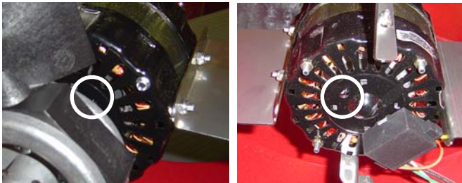
Figure 8: Oil hole locations. Access the oil holes by removing the protective grill(s) and turning the unit upside down.
