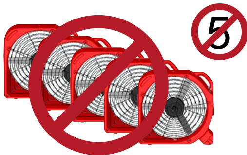
Figure 1: Too many AXIAL AIR MOVERS daisy-chained.
